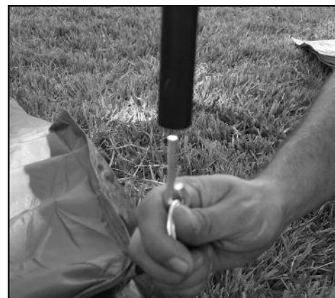
STEP 8 - Insert the pin located at the bottom of the arbor skin into the bottom of the pole to secure legs.
