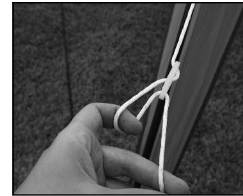
STEP 14 - Pull the bottom section looped in the clew out. The knot will not let the rope slip out.
