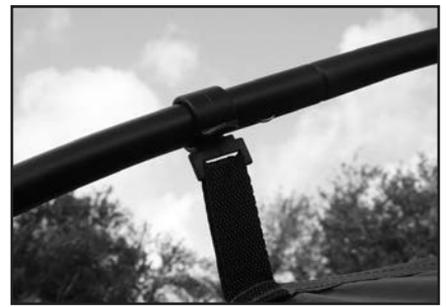
**Step 11 - Attach the speed clips to the frame.**
