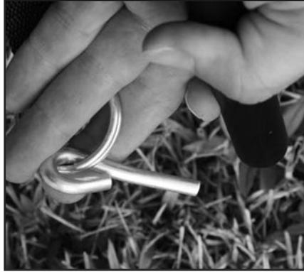
**Step 13 - Connect the last section of the leg poles and insert the pin and ring into the bottom of each leg pole.**
