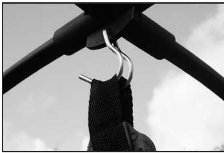
**Step 10 - Hook the web loop onto the molded roof joint.**
